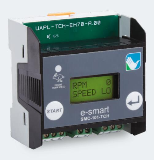
A Tachometer is a sensor device for measuring the rotation speed of an object such as the engine shaft in a car. This device indicates the revolutions per minute (RPM) performed by the object. The Uni-tech e-smart SMC-101-TCH is microcontroller based Tachometer with LCD display and OVERSPEED Fault indication LED. It is frequency measurement device that calculates speed by measuring the frequency of the incoming pulses.
