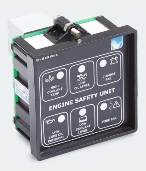
The Uni-tech e-smart ESU is microcontroller based Engine Safety Unit (ESU). The control provides a simple operator interface to the Engine with EMG / AUX. STOP control, shutdown Fault indication by LED and buzzer .The unit finds application in Engine automation panels of all complexities.
