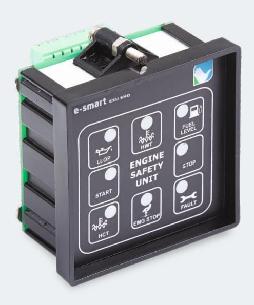
The Uni-tech e-smart ESU-SHD is microcontroller based Engine Safety Unit (ESU). The control provides a simple operator interface to the Engine with EMG / AUX. STOP control, shutdown Fault indication by LED and buzzer .The unit finds application in Engine automation panels of all complexities.
