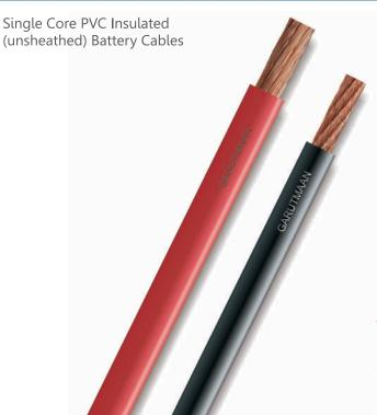
"Garutmaan" Single Core PVC insulated (unsheathed) battery cables, are manufactured using high conductivity, electrolytic grade, bright, plain annealed copper conductors.
